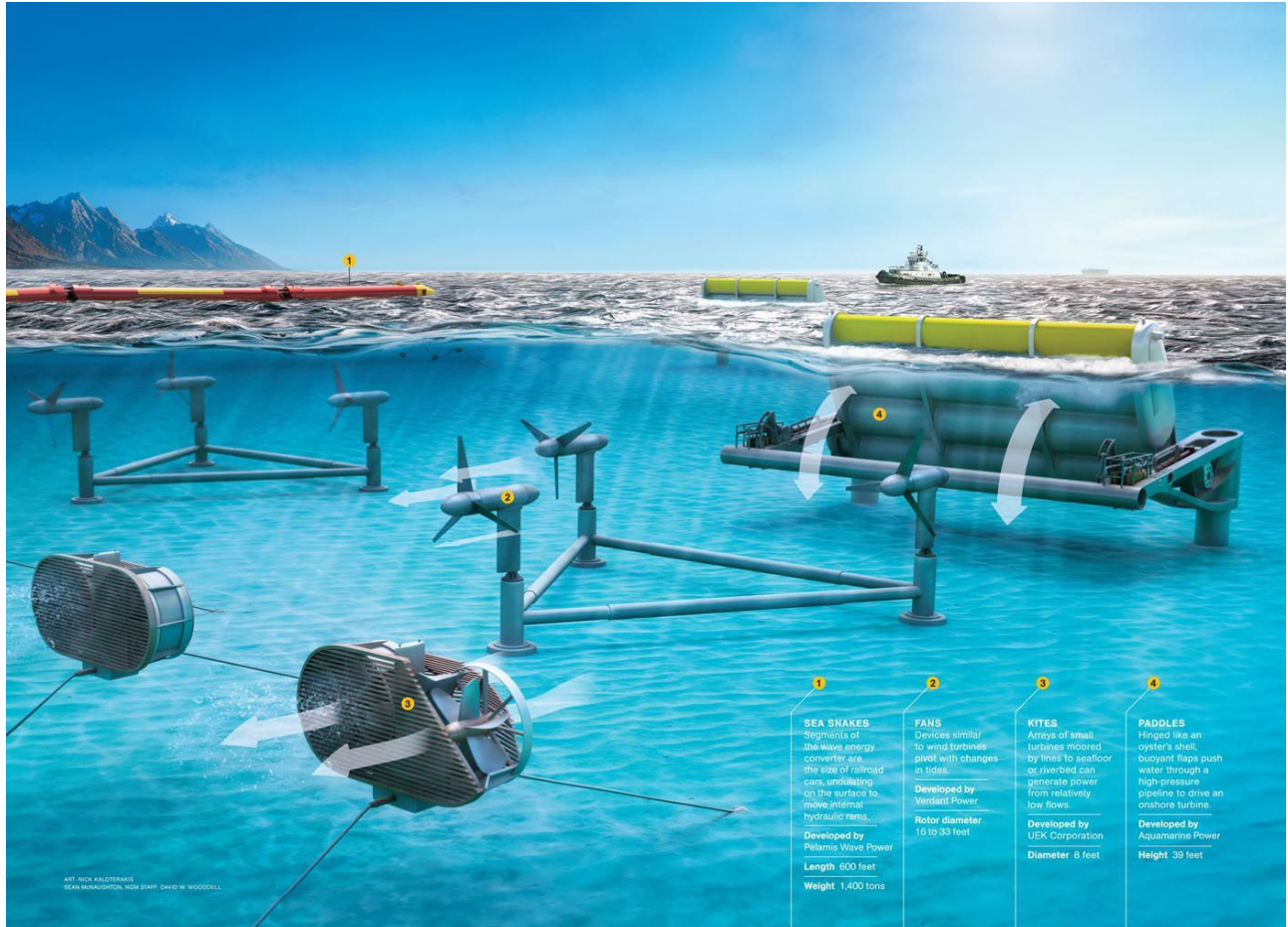
figure 7: This image depicts some of the methods used in collecting marine energy. (Top to Bottom) The first device is similar to the Pelamis and captures the power of the swells. The next one shows how waves might push the device down, generating energy. The next two show some turbines that generate power when water is pushed through them.
